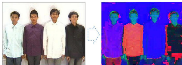
Fig. 9. Conversion of RGB to HSV color space of the input image.
