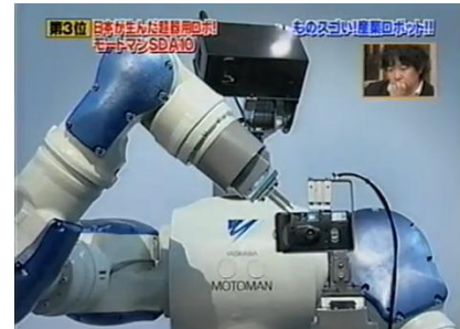
Fig. 12. Motoman SDA10 assembles a camera [30].
