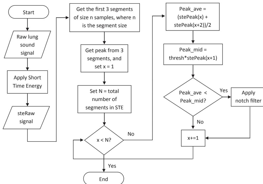
**Figure 3.** Joint Time-Frequency Denoising Flowchart for removing the mechanical noise in lung sounds
