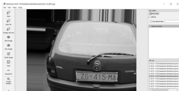
Fig. 8. LabelImg, the annotation tool used to annotate the images in the dataset
