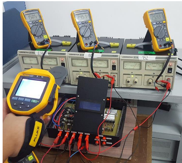
Fig. 7 Thermal testing set-up
