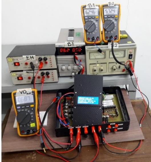
Fig. 2 Voltage monitoring testing set-up
