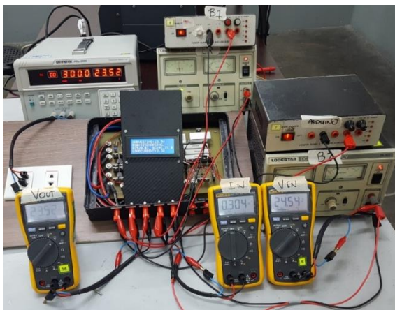
Fig. 6 Load detection testing set-up
