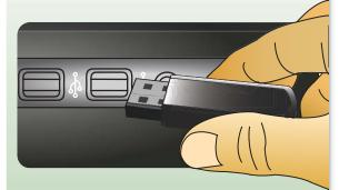
**Important:** After use, unplug USB receiver from thin client and attach it securely back into the wireless presentation remote.
