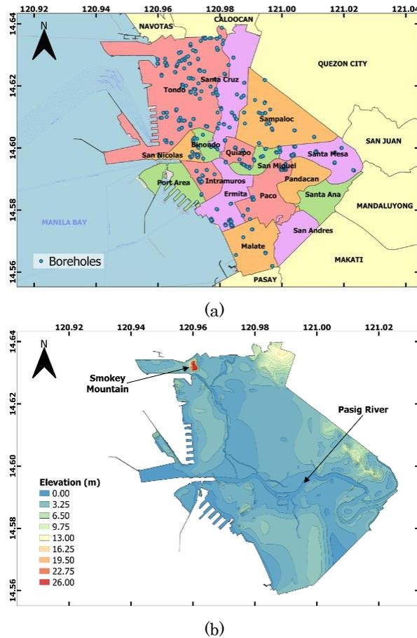
Fig. 1. (a) Geographical location of the City of Manila and the distribution of boreholes used in this study; (b) Contour map of the City of Manila with 1-m intervals.
