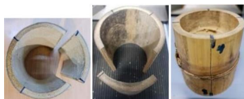
Fig. 3. Shear Failure Modes
