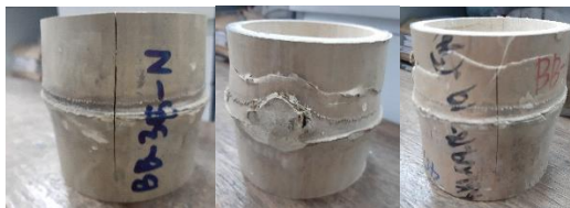
Fig. 2. Compressive Failure Modes
