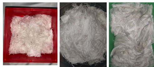
Fig. 1. Cut cotton fibers (10mm, 30mm, and 50mm from left to right, respectively).
