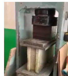
Fig. 1. Testing the compressive strength of Concrete.
