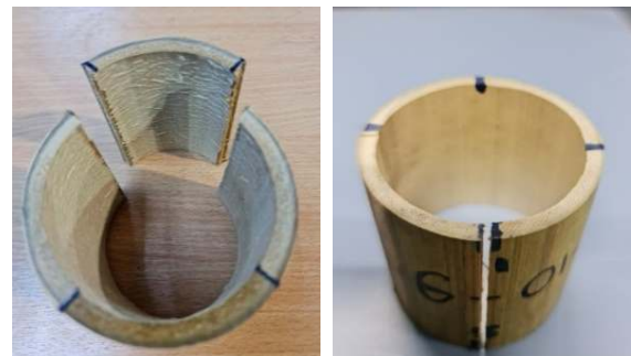
Fig. 3. Typical Shear Failure Patterns
