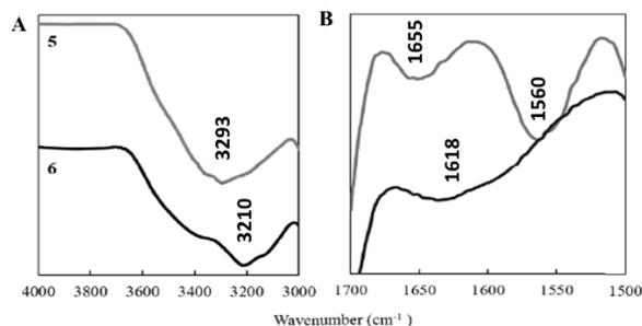
Fig. 3 Expanded FTIR spectra of bare EDA-f-PP-g-PGMA (5) and Pd-EDA-f-PP-g-PGMA (6)
