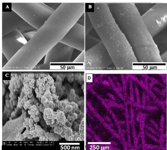
Fig. 5 SEM images of (A) EDA-f-PP-g-PGMA **5**; (B) Pd-EDA-f-PP-g-PGMA **6** with 6.0 mM initial Pd precursor concentration; (C) magnified SEM image (100K x) of **6**; and (D) Pd map surface of **6**. (Reproduced from Lopez, et al. 2020, with permission from Royal Society of Chemistry)
