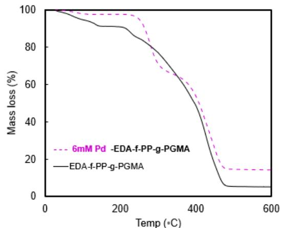
Fig. 6 Thermal profile of Pd-EDA-f-PP-g-PGMA using TGA
