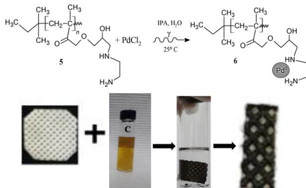
Fig. 2 EDA-f-PP-g-PGMA in 6.0 mM PdCl<sub>2</sub> before and after gamma irradiation
