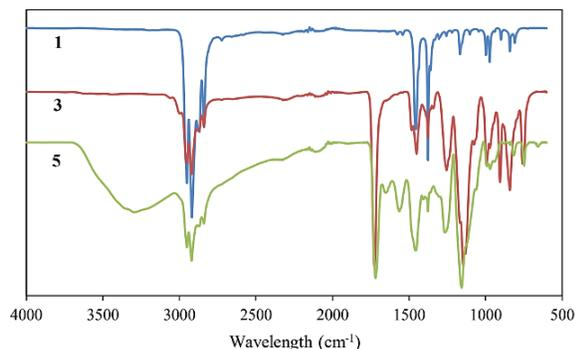
Fig.1 FTIR spectra of PP (1) PP-g-PGMA (3), and EDA-f-PP-g-PGMA (5)
