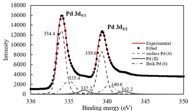
Fig. 4. HR-XPS spectra of Pd-EDA-f-PP-g-PGMA **6** irradiated at 50 kGy and 6.0 mM Pd precursor concentrations
