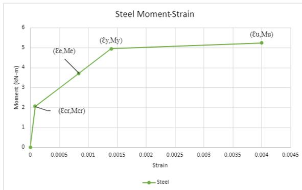
Fig. 4. Moment-strain diagram of steel reinforced concrete beam.
