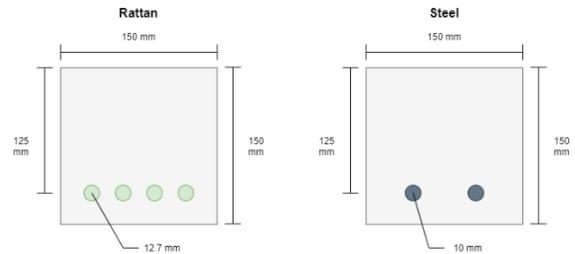
Fig. 5. Cross-section of rattan and steel used in the analytical flexural analysis.
