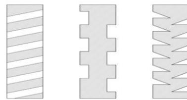
Fig. 2. Physical corrugations (from left to right): helical/spiral, hatches, and notches.
