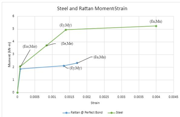
Fig. 8. Steel and rattan moment-strain plot.
