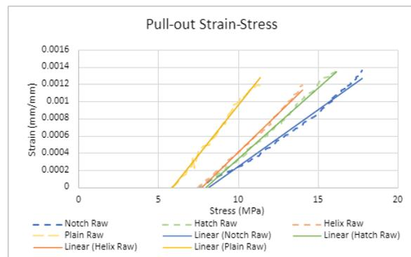
Fig. 7. Pull-out strain-stress data with linearized (solid) and raw (dashed) data.
