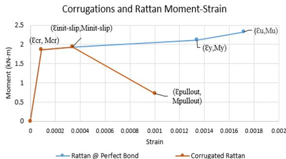
Fig. 6. Moment-strain diagram of rattan at perfect bond with concrete and rattan.
