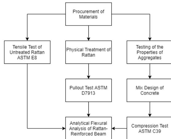
Fig. 1. Experimental procedure.
