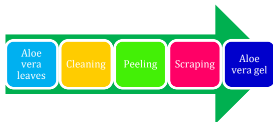
Figure 1: Flow chart for the production of Aloe vera gel
