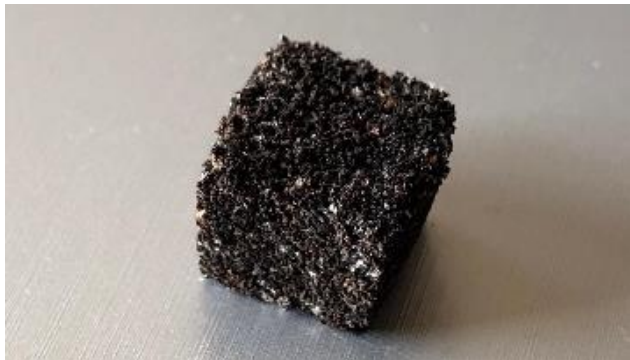
Fig. 5. Cube-shaped sample of the WCG-derived bioelastomeric foam.
