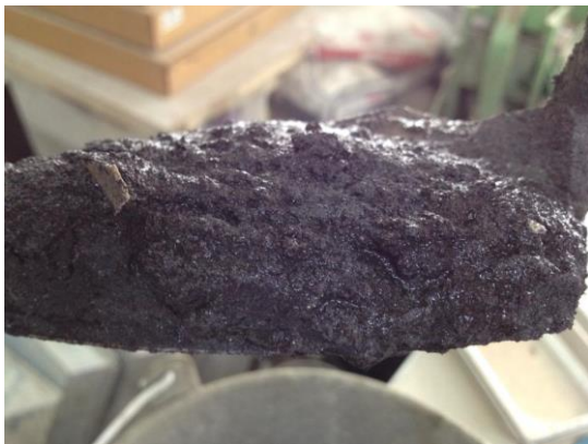
Figure 2. Metallic dusts mixed with water
