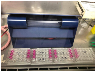
Fig. 2.2. P2, P3, P4, and P1 well plates arranged respectively. The exposed groups contain two sets of triplicates on each end while the control group contains one set of triplicate. Behind the well plates is the MOPA device.
