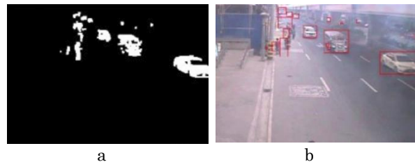
Figure 3: The Background Modeling and Removal process: (a) Image Binarization, and (b) initial selection of candidate vehicles via Blob Analysis
