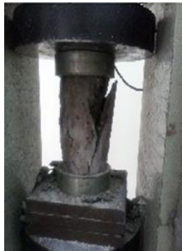
Figure 2 Mode of failure of cylindrical specimen
