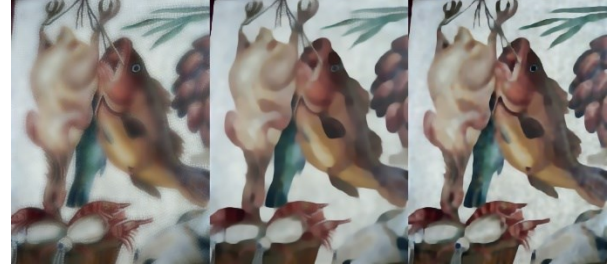
Fig. 3. Comparison of the texture removal using the original guided filter (left), the AnisGF (centre), and the SPGF (right).
