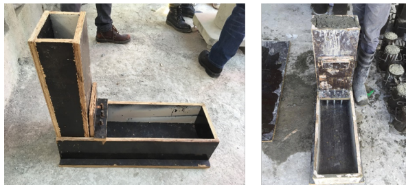
Fig. 3. Photo of L-box used, side view and front view
