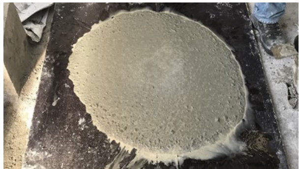
Fig. 1. Photo of slump flow within 600 to 900 mm
