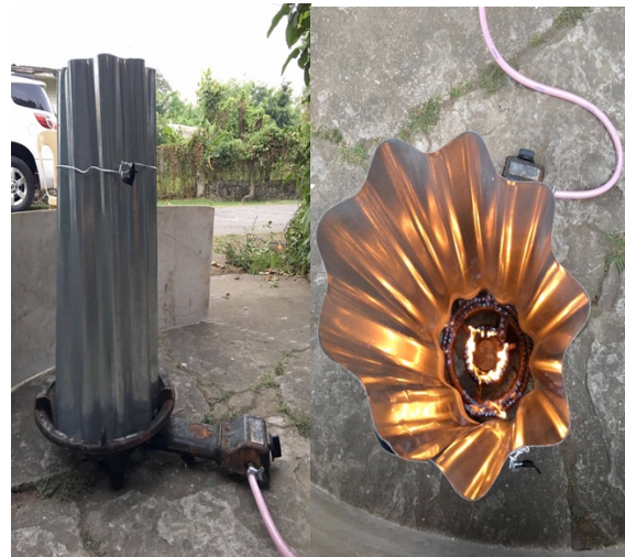
Fig. 3. Makeshift Chimney for the Burner
