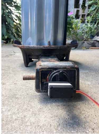
Fig. 4. Servo Motor Attached to the Flame Control Knob of the Burner
