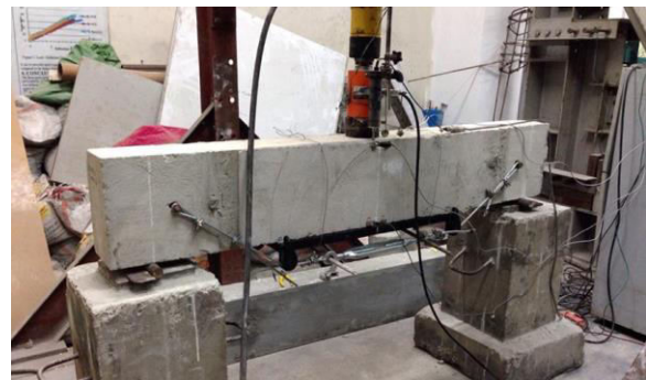
Fig. 5. RC beam test setup with T-EPT system
