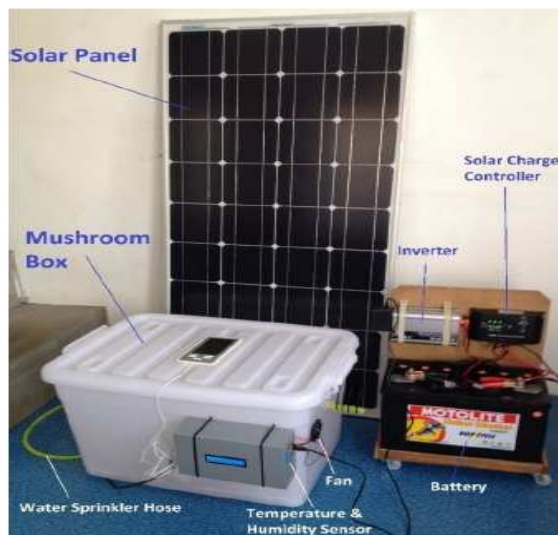
Figure 1. The complete setup for the controlled environment plant box
