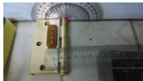
Figure 2. The apparatus used in determining the Roll-Off angle.
