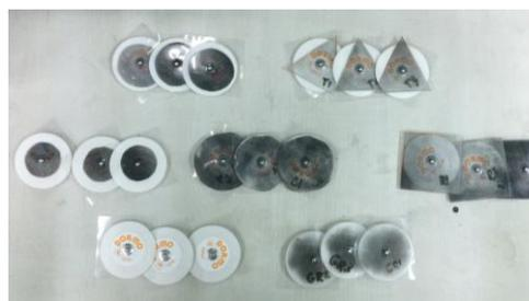
Fig. 2. The graphene samples labeled and attached in the medical electrodes.
