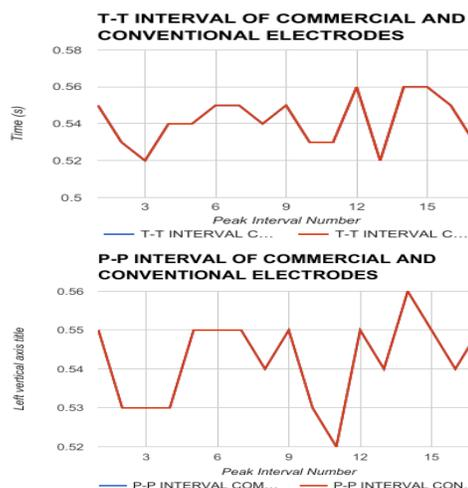
Fig. 4. The time intervals of the conventional and commercial graphene electrodes between their P and T waves.
