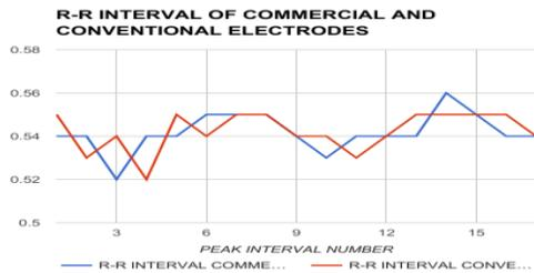
Fig. 5. The time intervals of the conventional and commercial graphene electrodes between their P and R waves.
