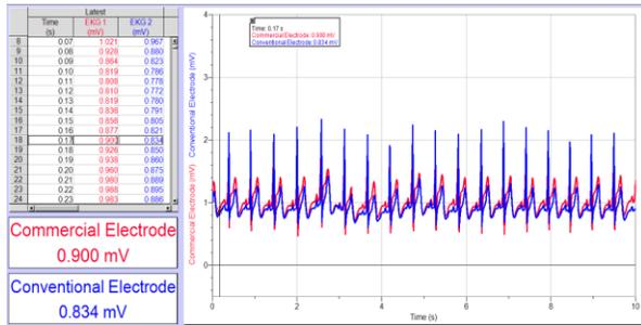
Fig. 3. ECG peaks recorded from the LoggerPro software.
