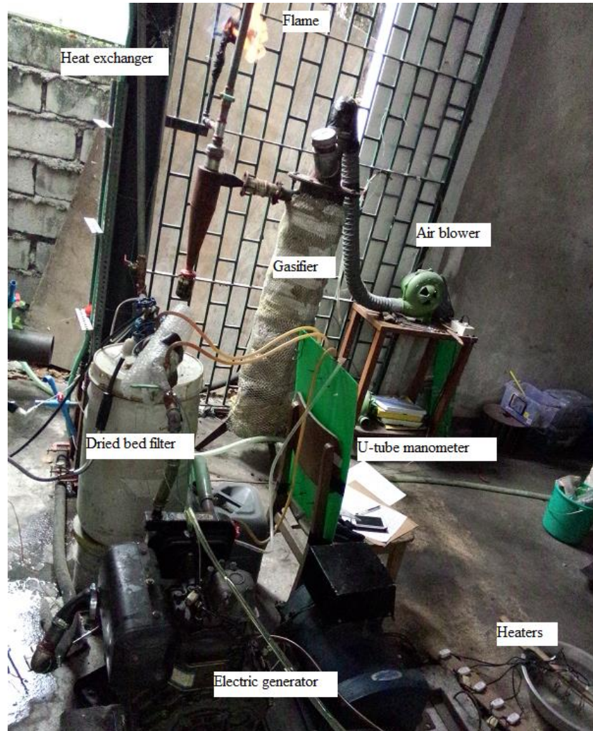
Fig. 1. Experimental apparatus of the gasifier-genset system
