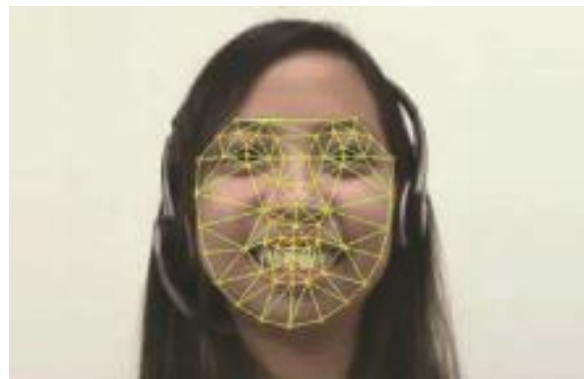
Fig. 2. 170 facial point distances computed from the 68 facial points
