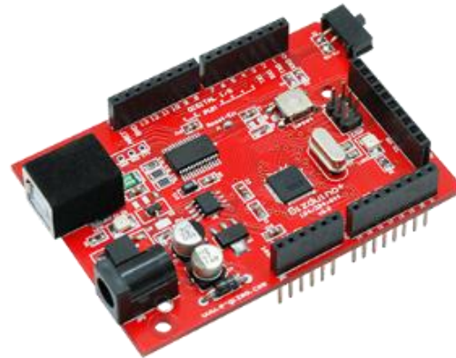
Figure 2.4 is the main component of the system where the data is being processed. Arduino served as a controller and identify whether the inputted plate number is a regular or a visitor on the institution.
