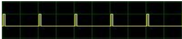
Figure 3.7 Duty Cycle from Controller Board (1)
