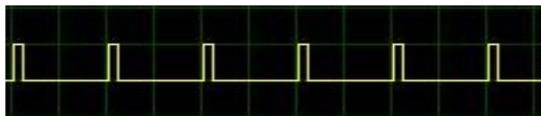
Figure 3.8: Duty Cycle from Controller Board (2)
