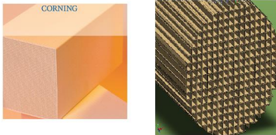
Figure 3: actual celcor ceramic (Corning) and solid works representation of stack
