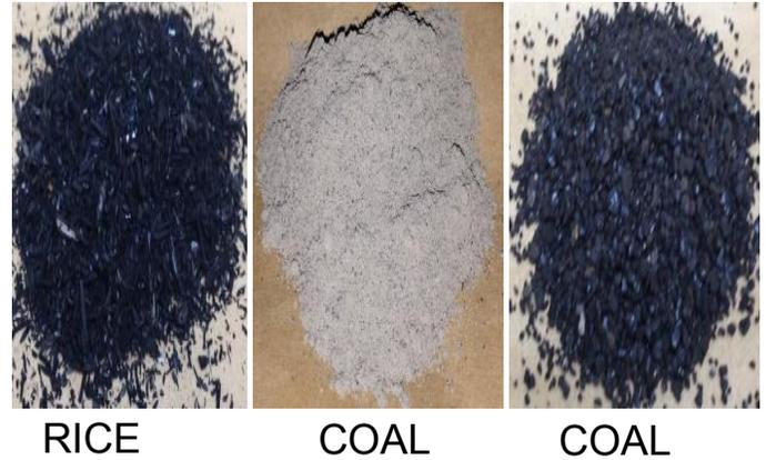
Fig. 1. Precursor materials used in the ternary mix geopolymer.
