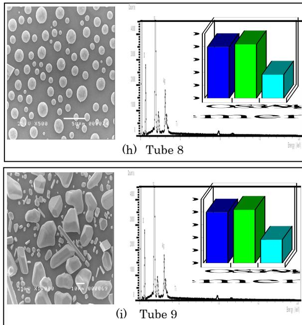
Figure. 2. Shape and EDX graph of micro- and nano-composite material typically in each tubes
