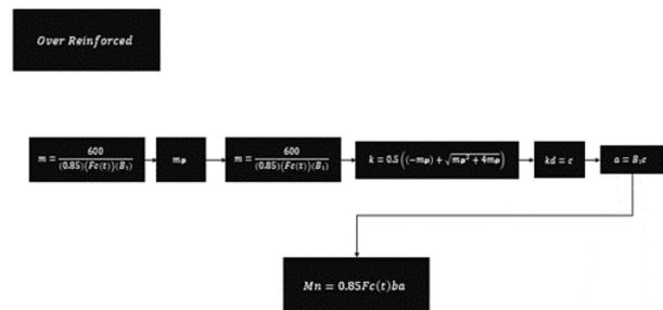
Fig. 4. Over Reinforced Case
