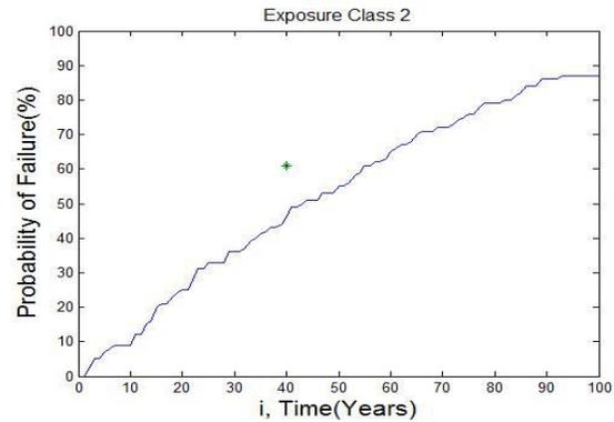
Fig. 8. Filtered Probability of Failure of Bridge 1
