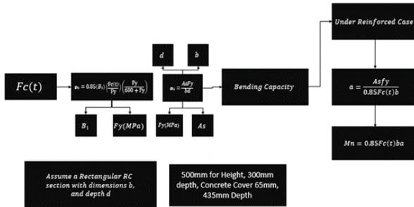
Fig. 3. Under Reinforced Case
