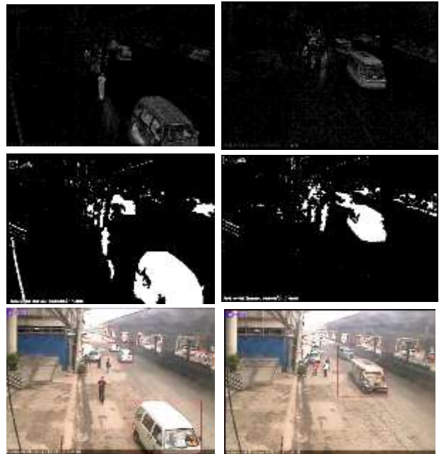
Figure 4 Top to bottom: image from traffic video, background image, subtracted image, subtracted image after morphological operations, image with counted vehicles.
