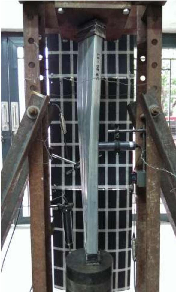
Fig. 2. Concentric compression loading of specimen showing buckling failure
