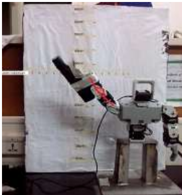
Fig. 9. Hand Wave Motion Data Experiment Setup of the Robot (Range: +10\text{m/s}^2 to -25\text{m/s}^2 )
