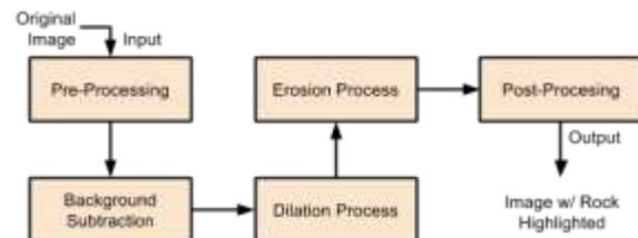
Fig. 1. Block Diagram of AVROWS Process
