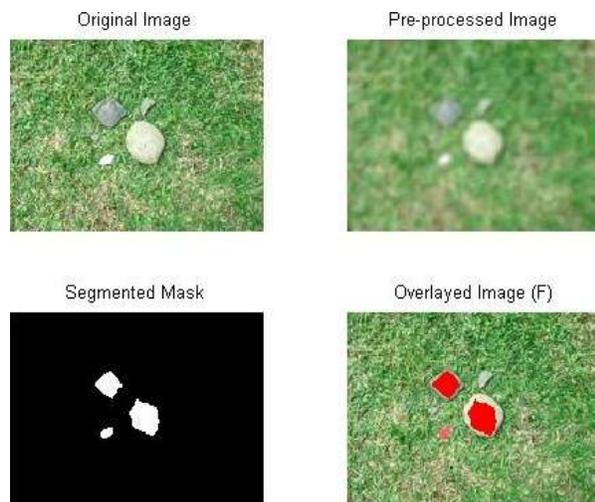
Fig. 8. Simulated landing shots taken at 1 meter (segmented and overlaid)
