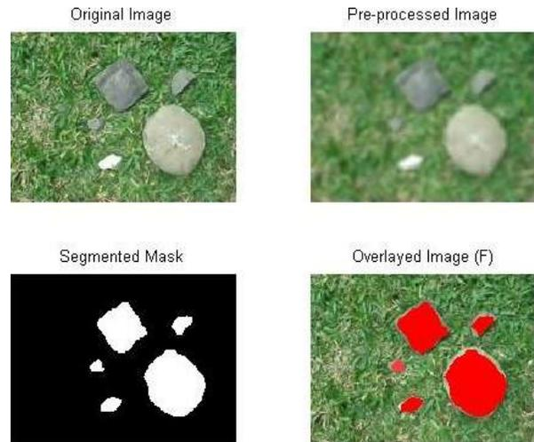
Fig. 9. Simulated landing shots taken at 0.5 meter (segmented and overlaid)
