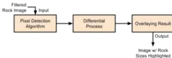
Fig. 3. AVROWS Post-Processing Block Diagram
