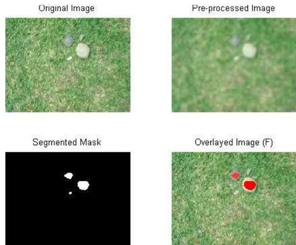
Fig. 7. Simulated landing shots taken at 1.5 meter (segmented and overlaid)
