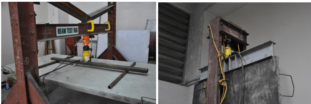
Figure 3. Actual Set-up of Test for Transverse Load Test (left) and Axial Compressive Load Test (right)
