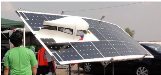
Figure 1. Sikat 2 solar array
