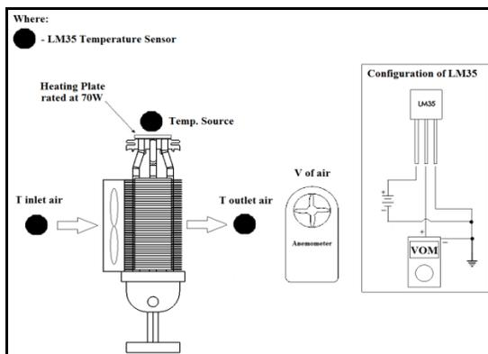
Figure 1 Test Setup Schematic
