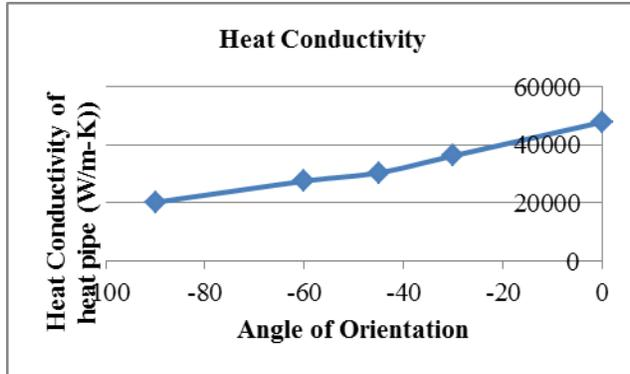
Figure 4. Heat Conductivity of the heat pipe with respect to orientation
