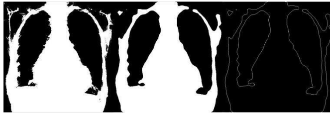
Figure 5. Visual Definition of an (a) Original Image in Binary, (b) Image using Disk Filter, and (c) Image using Laplacian Filter
