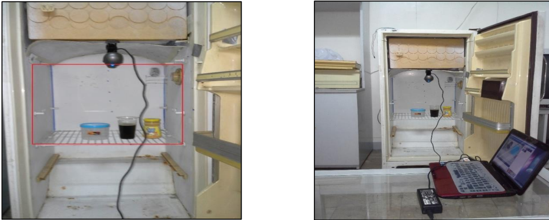
Figure 1. Area of interest marked in red (left) and Physical setup of the system (right).
