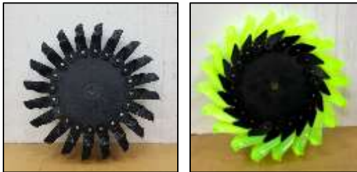
Fig. 10. Pelton wheel with Traditional buckets and PET buckets
