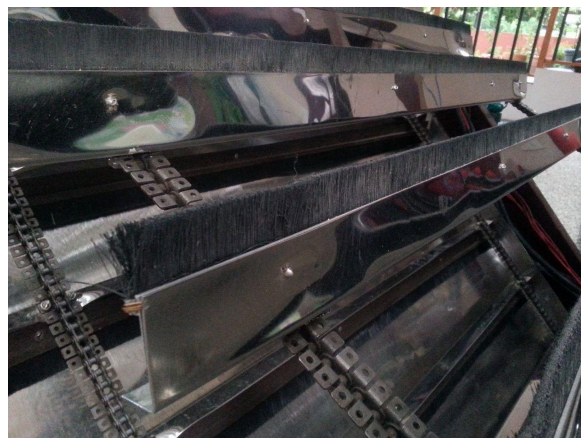
Fig. 6. Stainless Steel L-bars with brush strips
