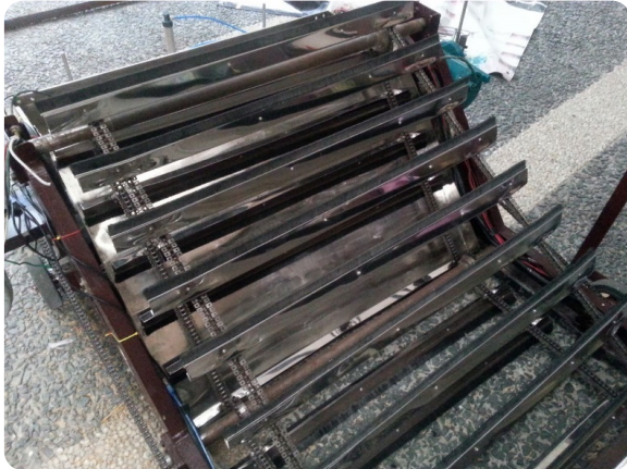
Fig. 7. Sweeper wheel design mounted on a mobile robot frame
