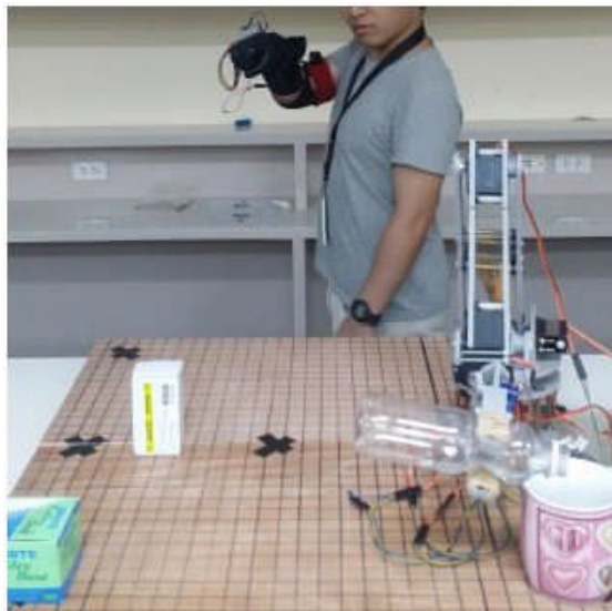
Fig. 3.2 Overall Operation of Glove Controller and Robotic Arm Setup
