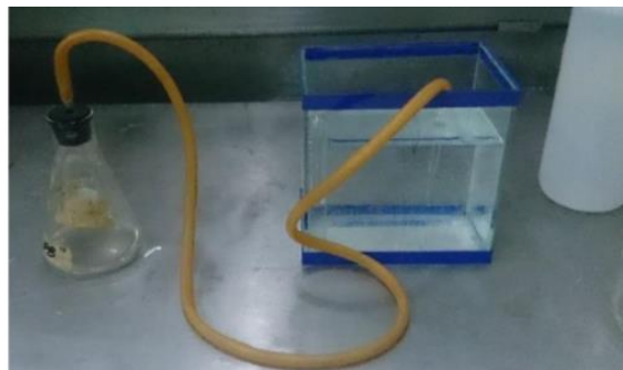
Figure 1. Set-up for the fabrication of Hydrogen Sulfide (H 2 S) gas
