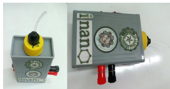
Figure 6: Sample of the fabricated prototype metal-oxide nanosensors.
