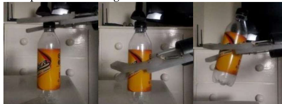
Figure 10. Bottle Lifted by Prosthesis
