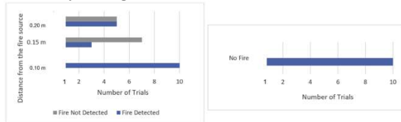
Fig. 7. The YG-1006 sensor's data regarding the detection of infrared levels
