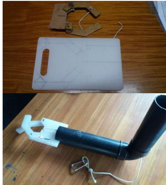
Figure 3-4. Cardboard Prototype of Claw Gripper and Final Prototype with Claw Gripper and Arm
