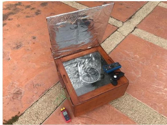
Figure 5 Cooking Power Test Experimental Set-up
