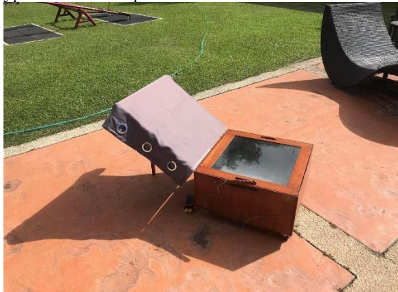
Figure 4 Stagnation Temperature Test Experimental Set-up
