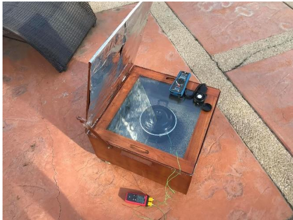
Figure 6 Rice Cooking Test Experimental Set-up
