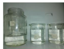
Figure 5. Swelling Test of Synthesized Mung Bean based Bioplastic in Different Solvents
