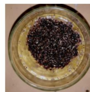
Figure 8. F5 bio-adsorbent, after 4 hours contact time
