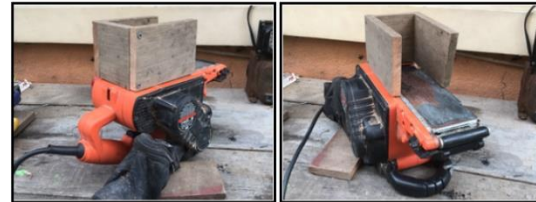
Figure 2. Abrasion Resistance Test Setup
