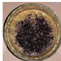
Figure 6. F3 bio-adsorbent, after 4 hours contact time
