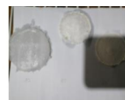
Figure 6. Residue of Bioplastic film after Swelling Test
