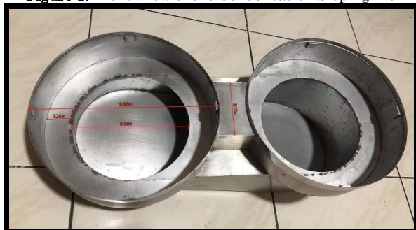
Figure 2. Bottom View of the Condensation Sloping Lid
