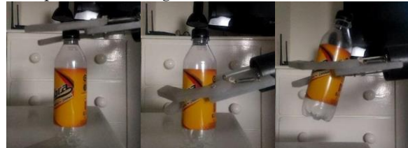
Figure 10. Bottle Lifted by Prosthesis
