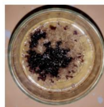
Figure 4. F1 bio-adsorbent, after 4 hours contact time
