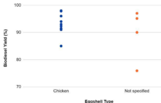
Fig. 3.6. Biodiesel Yield of Eggshell-Derived Catalyst
