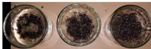
Figure 3. Set-ups after placement of bio-adsorbents F2 (left), F3 (middle), and F4 (right)
