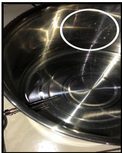
Figure 9. Condensed Water Droplets on the Unsubmerged Wall of the Container
